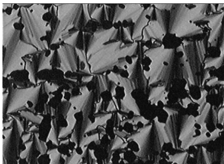
Fig. 2 The textural change obtained for the transition from the ferroelectric phase to the unidentified isotropic phase on heating for the homogeneously aligned sample of compound I , where the texture of the unidentified isotropic phase appeared as lots of round shaped dark domains.
