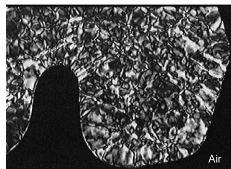
Fig. 1 The texture obtained for the ferrielectric phase of compound I (145 °C).
